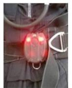
distress signal unit with lights activated in full alarm.
