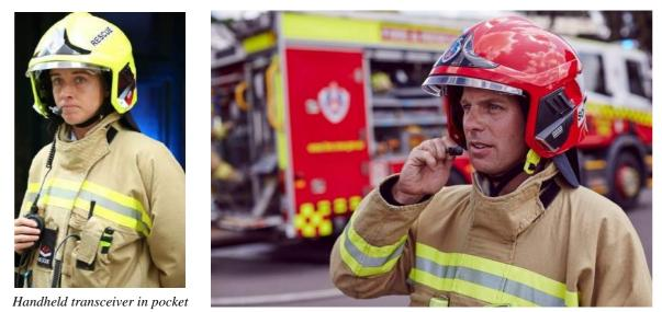
Figure 41 Handheld transceiver, and structural helmet speaker and microphone
