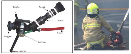
Monitors are used to deliver large quantities of water while avoiding the need to manually hold and direct the hose.
