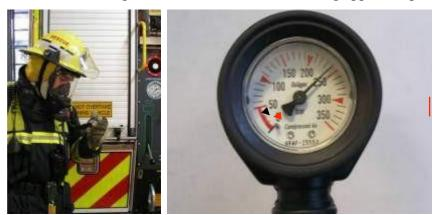
Self contained breathing apparatus cylinder pressure gauge (hand held). An alarm sounds when the pressure is low.
